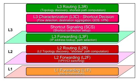
L3C performs an analysis of the type of traffic that is being handled and makes decisions as to how packet forwarding is to be accommodated. In the case of TAG/MPLS, the topology routing structure that was created in the L3R function is used to define a connection. SCS performs the streamlined connection setup functions. For TAG switching, it uses the Tag Distribution Protocol (TDP).
