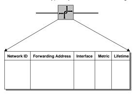
Figure 5. Routing table structure
