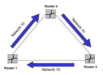
Figure 6. An example of a routing loop.
