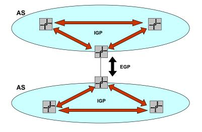
Figure 9. Autonomous systems, interior gateway protocols, and exterior gateway protocols .
